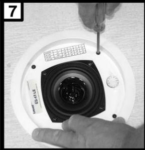
For use in a speaker system without using the internal matching transformer, one cable should run from the output of an 8 ohm maximum 25 watt amplifier to one ES-4T-LE speaker only, or from the output a 4 ohm maximum 50 watt amplifier to one ES-62T-LE speaker only. Wiring the speaker system in a series/parallel configuration may be acceptable depending upon the amplifier used, but that wiring method is not covered in this installation manual.
