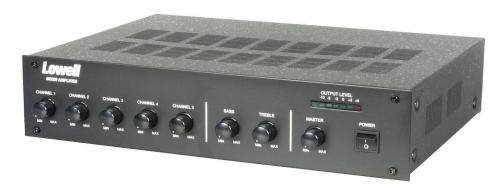
Rackmount mixer with 250W amplifier is powered via switchable 115 or 230 VAC @ 50/60Hz or 24VDC. Includes five channel volume controls, treble and bass controls, master volume control, main power switch, and LED display bank for output level.
