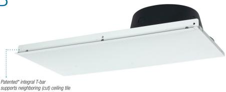
LT SERIES SPEAKERS are pro systems made for quick installation in suspended lay-in tile ceilings. This model features an 8-inch 15W dual cone driver, 25V/70V dual voltage transformer, 1x2 white grille with black subplate and 0.147 cu.ft. enclosure. The patented\* 1x2 assembly features an integral T-bar support that replaces one-half of a 2x2 or one-fourth of a 2x4 ceiling tile.
