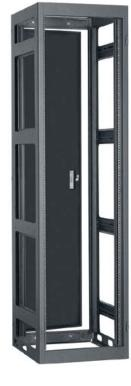
Gangable rack with adjustable rails is fully welded 16-gauge steel with 14-gauge base, reinforced at all load-bearing junctions.
