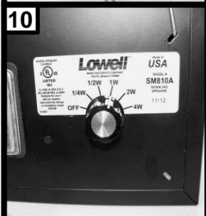
**10** A transformer tap selector switch is provided on the side of the masking speaker enclosure. “OFF” and 70V 1/4W, 1/2W, 1W, 2W, and 4W select positions are provided. The transformer tap switch is set at 1W when shipped from the factory. Set the selector switch as specified by the system designer.
