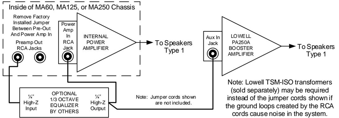
Connection to two (2) 1/3 octave equalizers using Lowell PA250A booster amplifiers with similar and different types of loudspeakers. (Note: Similar speakers are fed by the same equalizer).
