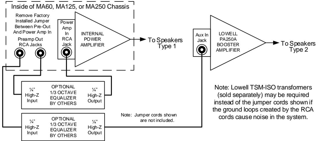
Connection to three (3) 1/3 octave equalizers using Lowell PA250A booster amplifiers with similar and different types of loudspeakers. (Similar speakers are fed by the same equalizer).
