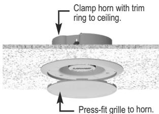
**Masonry:** 10.5" sq. x 4"D stainless steel backbox mounts into masonry wall. LUH-TP trim plate screws to backbox. Horn with trim ring clamps to trim plate (trim ring covers screws). Grille press-fits to horn assembly.
