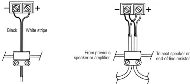
Model LUH-15T ships ready for hookup with a 2-conductor cable exiting through a rear cable clamp.
