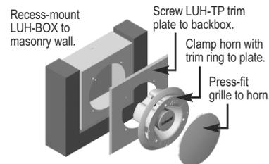
**Surface-mount:** 10.5" sq. x 4"D stainless steel backbox surface-mounts to wall. Horn with trim ring clamps to box (ring covers unused screw holes). Grille press-fits to horn assembly.
