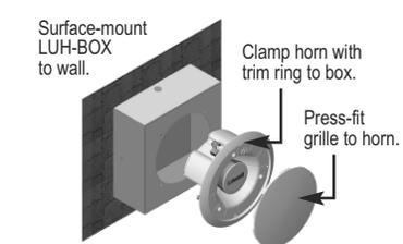
**Other Installation Accessories (not evaluated or approved by UL):** the UNIHORN® also features standard screw holes that fit the LUH-VRG vandal-resistant grille or any standard 8" speaker grille; however, these options have not been evaluated by UL. The LUH-VRG installs with spanner-head screws and screwdriver. Standard grilles screw-mount to the UNIHORN® and fit various backboxes. See individual product spec sheets for more information on standard 8" speaker grilles and backboxes.
