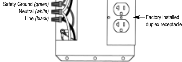
ACSP2004 wiring using only factory-installed receptacle
