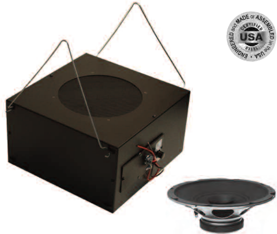
Model SM810RS (shown here) includes a rotary switch to adjust transformer taps. The SM810 speaker assembly includes a 700 cu.in. acoustic-lined backbox with perforated grille area, 8" 15W dual-cone speaker and pre-mounted wire hanger with chain and S-hooks for fast installation.
